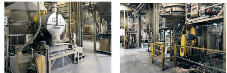
These Munson Rotary Batch Mixers have been in near-constant use since 1983. Records for the last 12 years show that one mixer has had 34 hours of downtime and the other just 4.5 hours.
