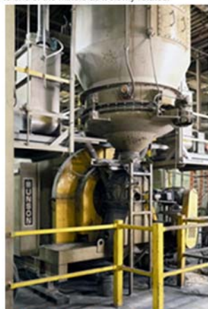
To fill the vessels, a pneumatic conveyor transports resins from compounding units to a holding hopper.
