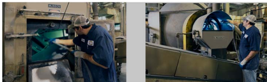
The hinged access doors at either side of the vessel provide access to all material contact surfaces for cleaning and visual inspection.
